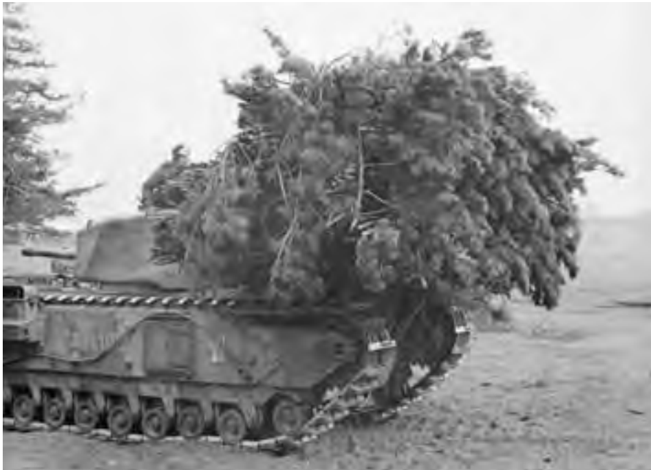
Figure 41. Fascine-carrying tank, Exercise Kruschen. (IWM H 29035)
