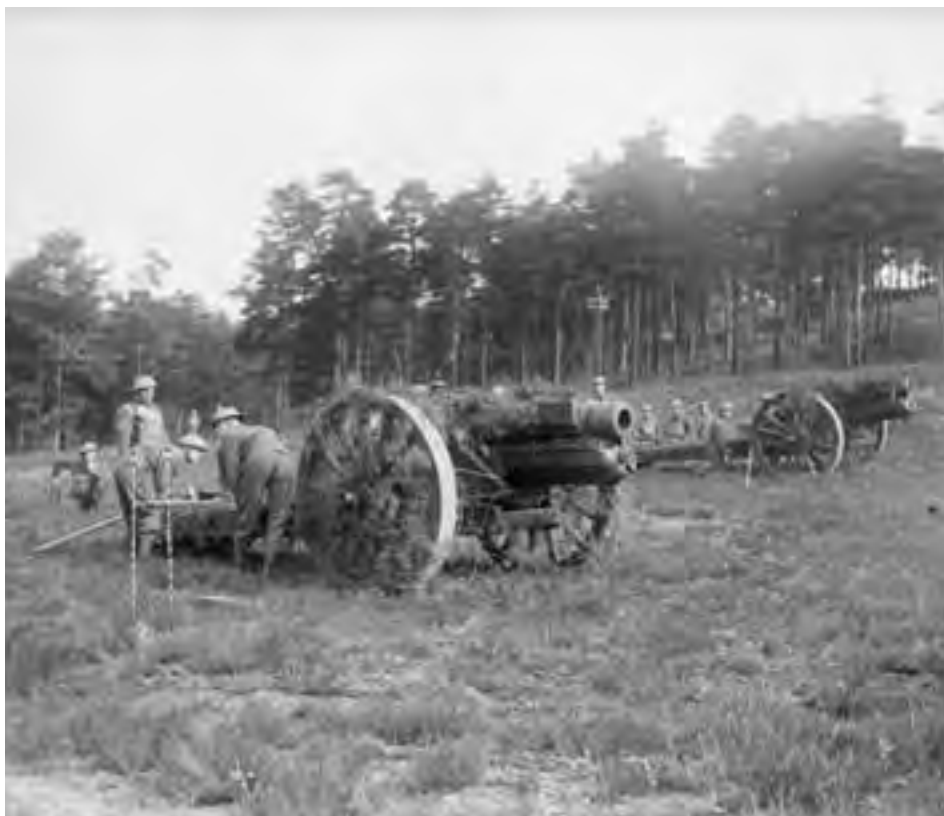
Figure 38. Photograph of a 6-inch howitzer taken somewhere in England, possibly Suffolk, in 1940. As with so much of the field artillery used for coastal defence, such guns were from the First World War and were taken out of storage in 1940. This example shows a gun in unmodernised form; over time they were refurbished and provided with pneumatic wheels. (Imperial War Museum H1248)
