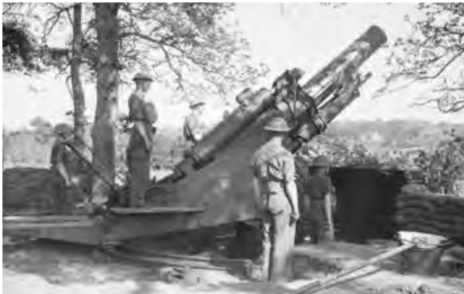
Figure 41. A 9.2-inch howitzer in Kent in 1940. This behemoth of a weapon was developed during the First World War for shelling well-built German trenches, but was pressed into service again in 1940 in anticipation of invasion, when its huge shells were expected to wreak havoc amongst a German landing fleet. (Imperial War Museum H1468)
